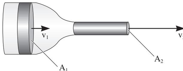
The terms  $A_1 v_1$  and  $A_2 v_2$  represent the **volume flow rate**  $Q$ , which is the volume of fluid that moves past a cross section of pipe in a given unit of time. These terms are represented in Figure#■ by two shaded cylindricals of equal volume. Since the tube has a lower cross sectional area on the right, the fluid passing through this constriction will have a larger velocity.
