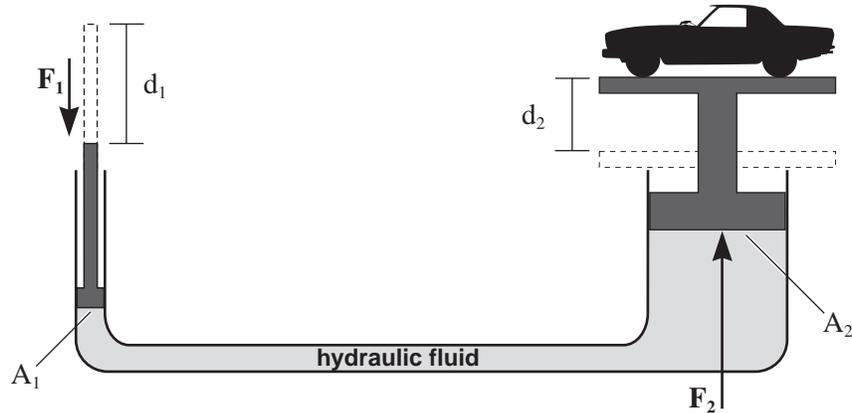
The force  $F_1$  is applied on the left end of the lift to a pistoned of area  $A_1$ . This creates an increase in pressure through out the fluid which is equal to  $F_1/A_1$ . At the right end of the lift this pressure acts on a larger cylinder with area  $A_2$ . Since the  $A_2 > A_1$ , it follows that  $F_2 > F_1$  :
