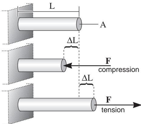
**Figure 7.1** Equal and opposite forces are present on both sides of the rod. To simplify this example, only the forces on the right side are shown.
